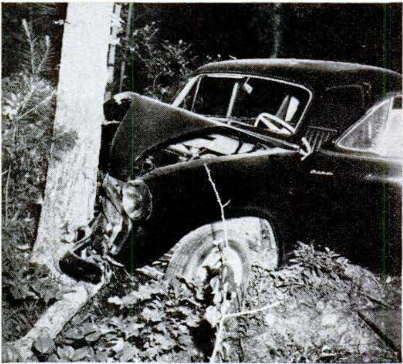
TREE did this to a Hillman that swerved to avoid a dog in the road, went out of control at 40 m.p.h. The tree, 10 inches thick, split.
